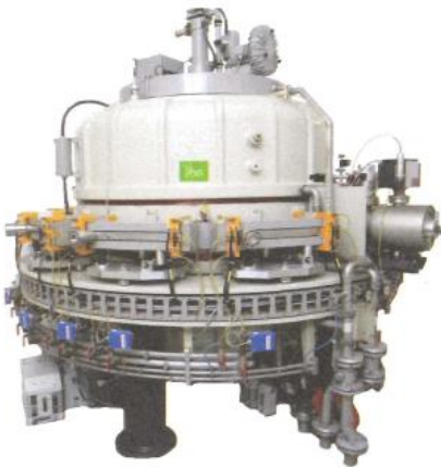
A Rhodotron, a commercial electron-beam accelerator for industrial applications including sterilization of medical devices
